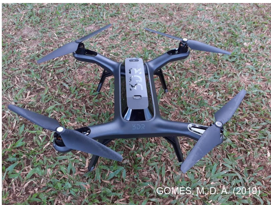
Figura 6 - Drone multirotor (SOLO – 3DR)
