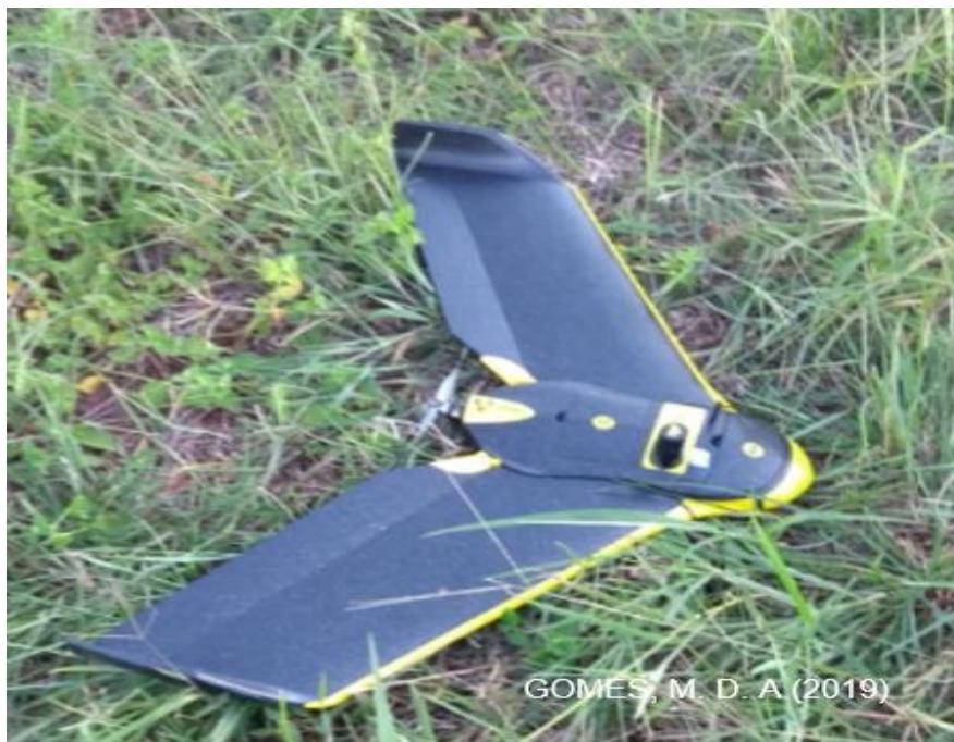
Figura 5 - Drone de asa fixa (eBee Plus – SenseFly)
